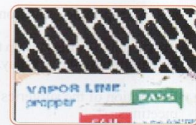
Bowie Dick test pack and vapor line indicator
